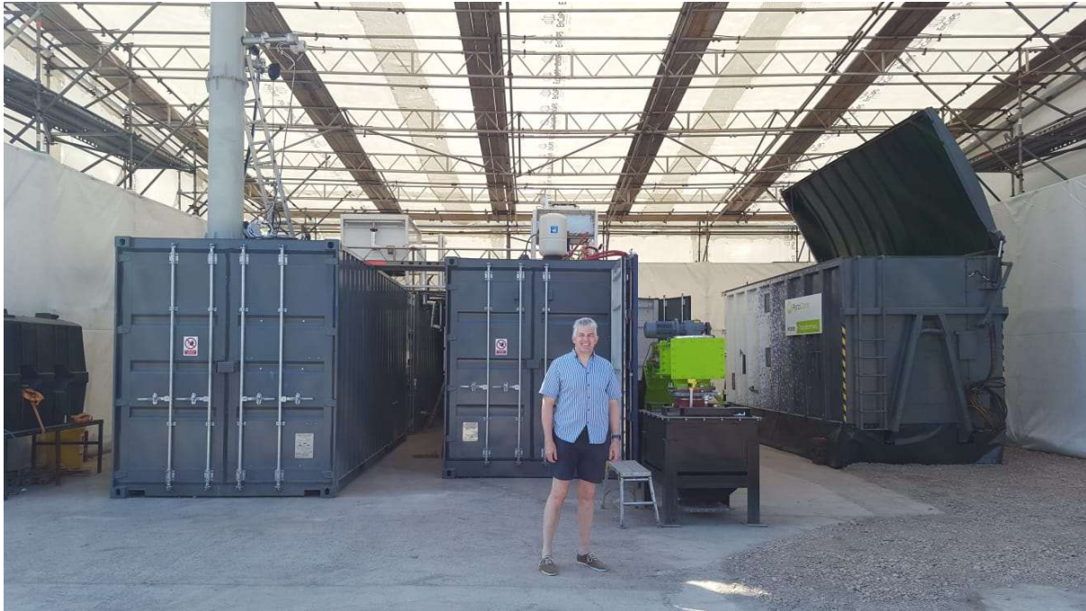
Figure 1. Pyrolysis kiln Demonstrator original layout, August 2019– 4 containers [L] and walking floor feed system [R]. Yes, that is myself
