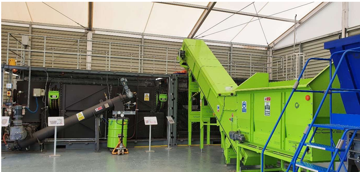
Figure 4. Coveya hopper and feed conveyor to feed hopper and Pyrolysis kiln, char cooling and recovery into barrels.
