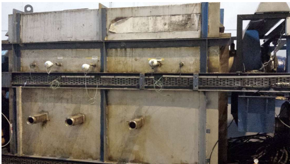
Figure 1. Pyrolysis kiln main body with burner view ports and thermocouples
