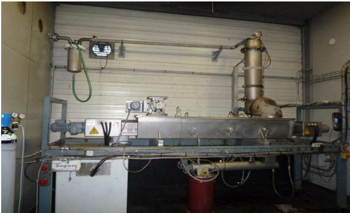
Figure 4. Biogreen/ETIA 10 kg/h electrically heated pyrolysis unit.
