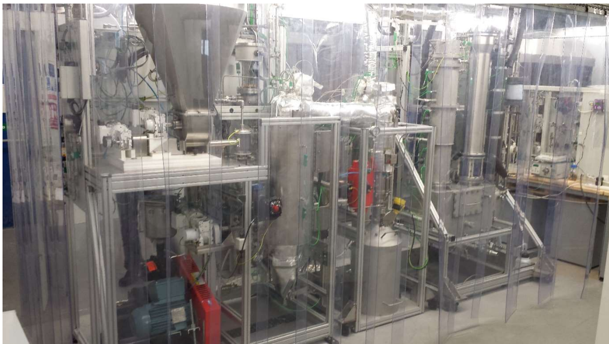
Figure 5. 5 kg/h fluid bed fast pyrolysis rig and liquids collection system
