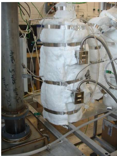
Figure 7. Lagged, heated HVF
