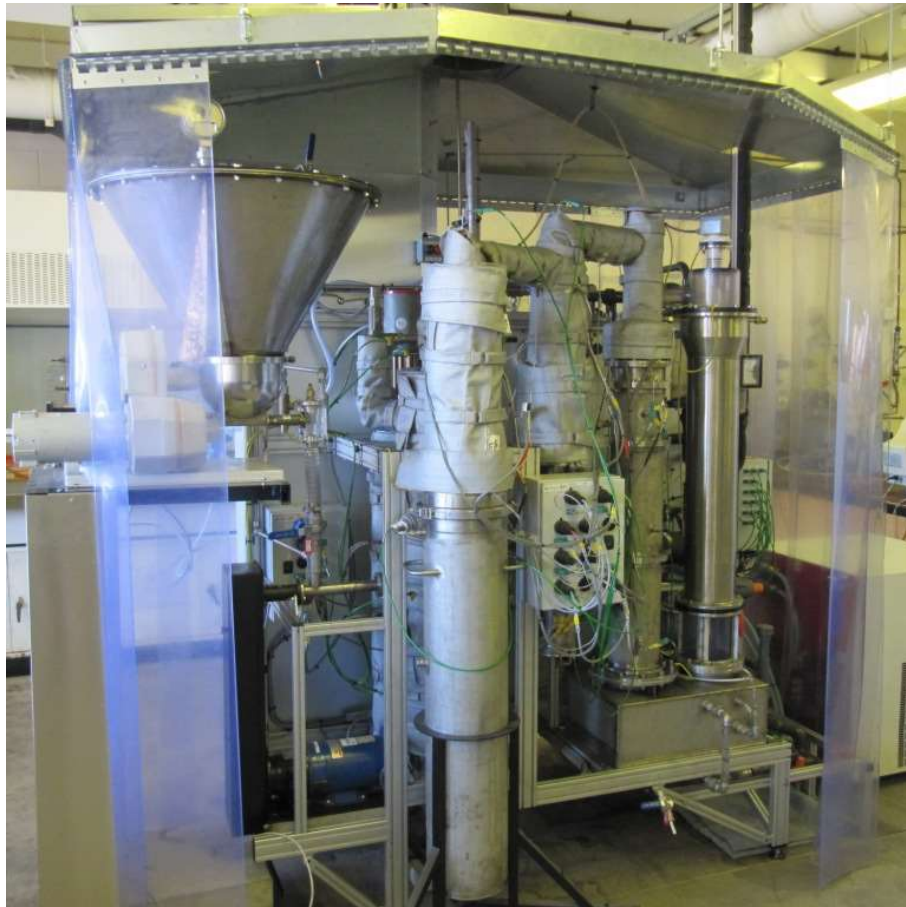
5 kg/h fluid bed reactor with clean gas recirculation [2010] after major upgrades and overhaul
