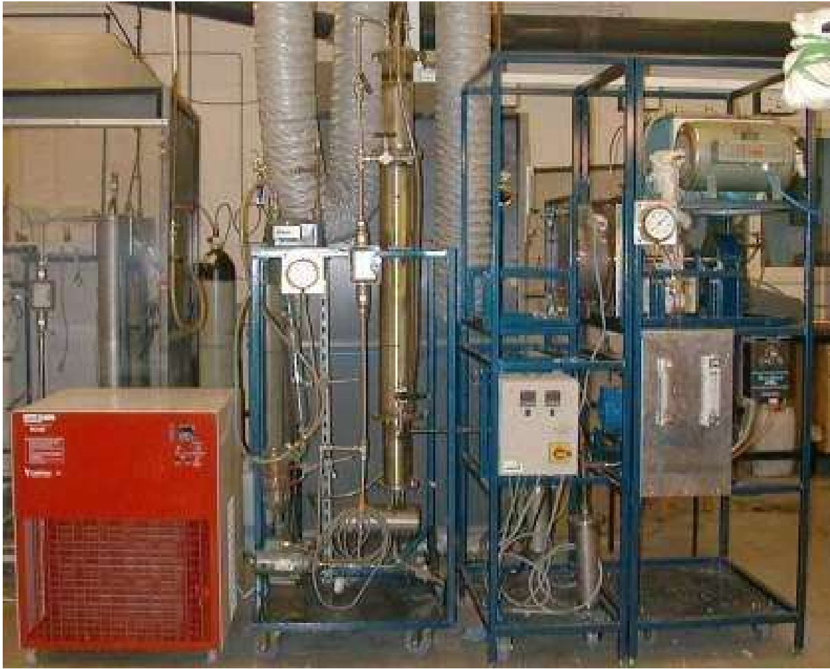
10-20 kg/h ablative pyrolysis rig. Version 2 [1997 build]
