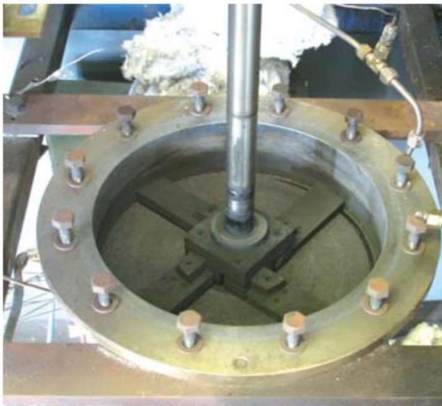
5 kg/h ablative pyrolysis rig, Aston University. Version 1. Rotating angled blades
