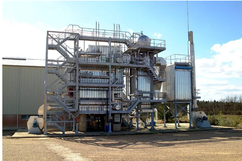
650 kg/h fluid bed combustor, 3.5 MW th input
