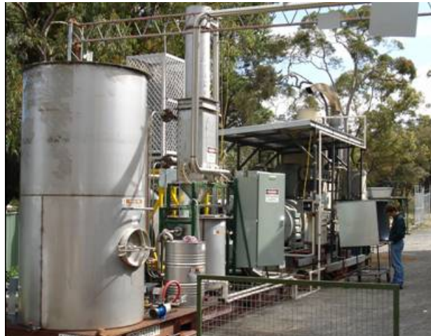
Biodiesel scrubber and 300 kWe gas engine, Gosford, Australia (2006)
