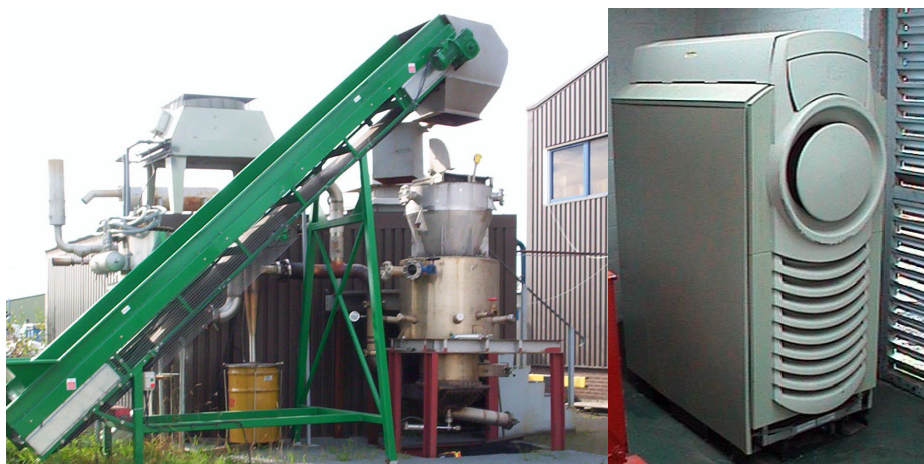
60-80 kg/h test gasifier
