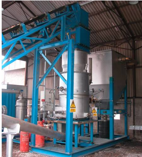
250 kg/h gasifier and hot gas filter
