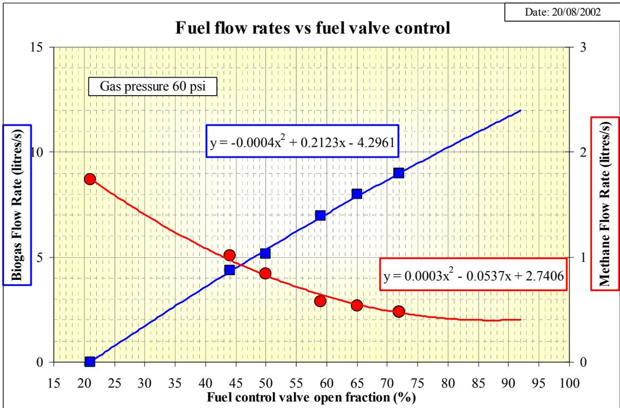
**Figure 15: Fuel Volume Flow Rates in Test 3**
