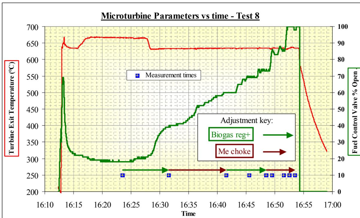
**Figure 31: Logged Microturbine Parameters During Test 8**
