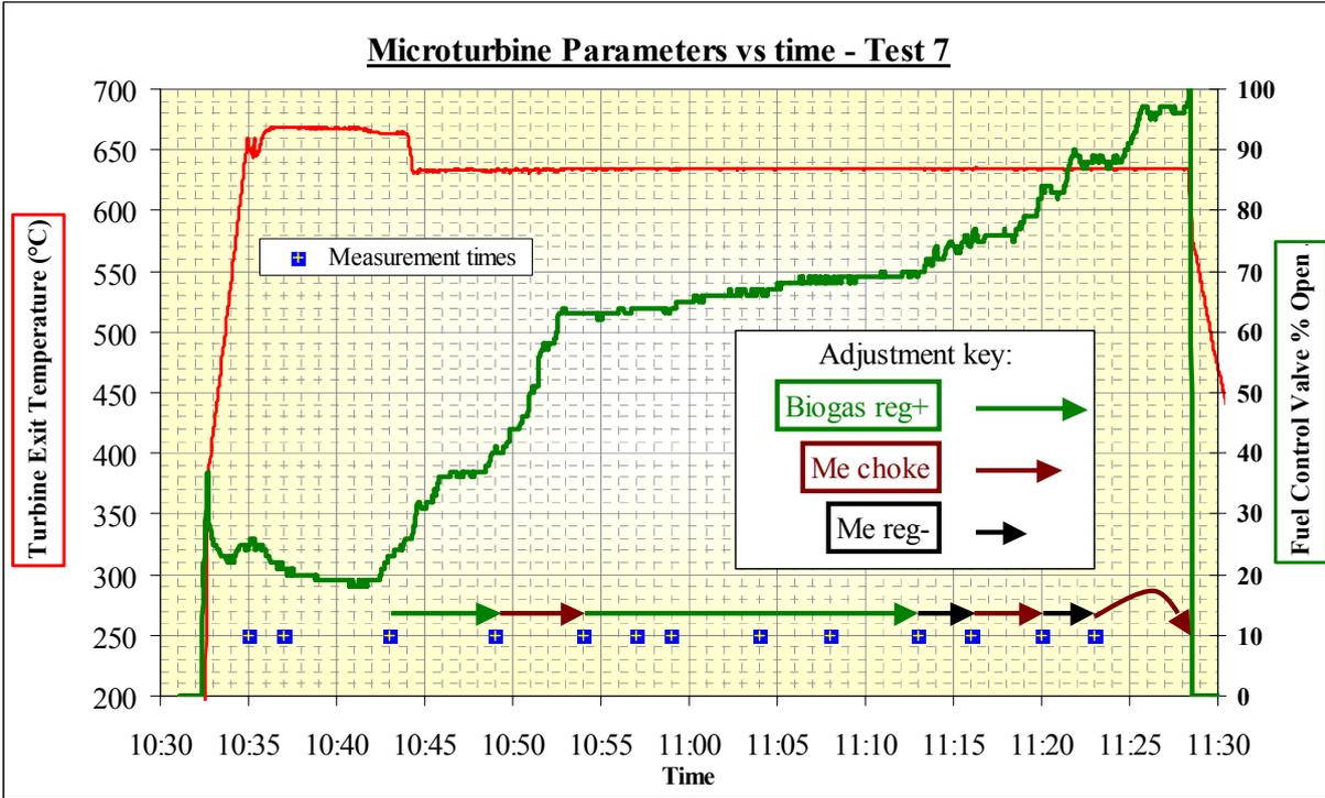
Figure 26: Logged Microturbine Parameters During Test 7
