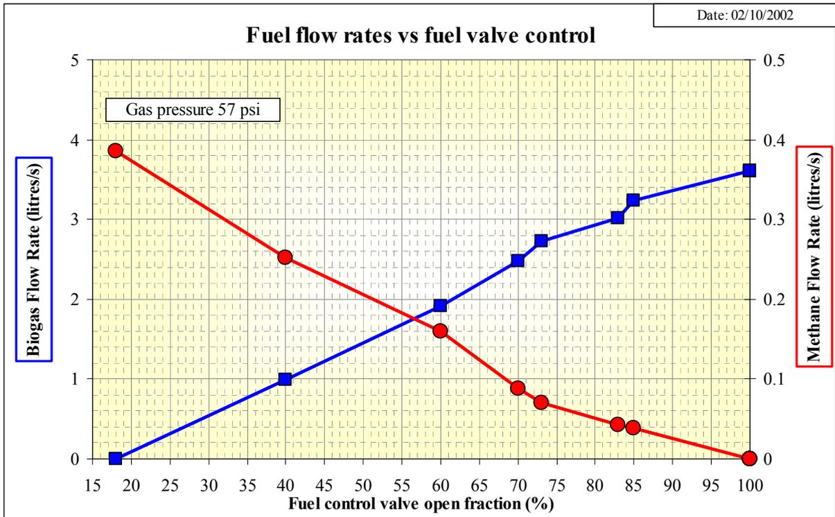
Figure 32: Fuel Volume Flow Rates in Test 8
