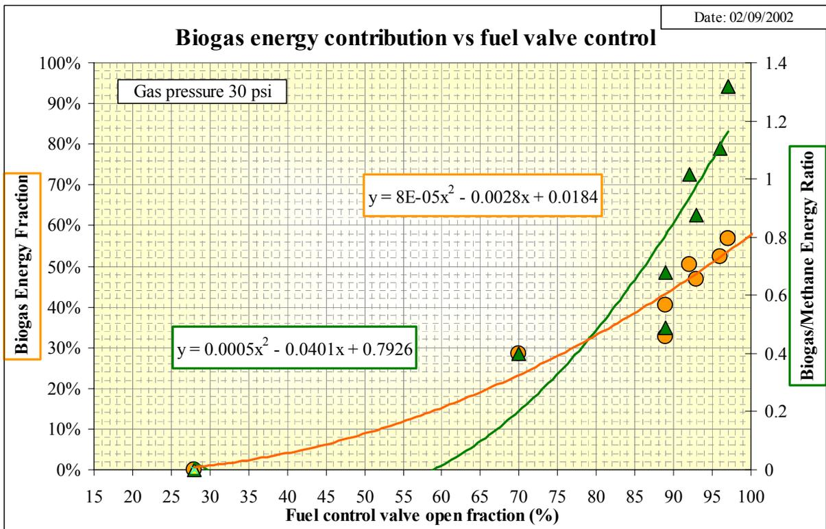
Figure 19: Fuel Energy Balance Analysis in Test 4
