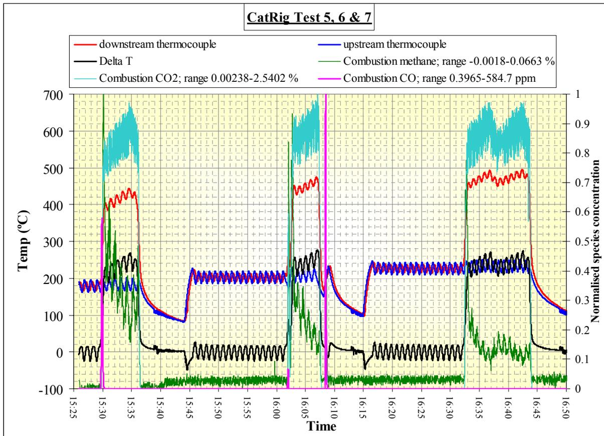
**Figure 42: Temperatures and gas species concentrations for CatRig Tests 5-7
