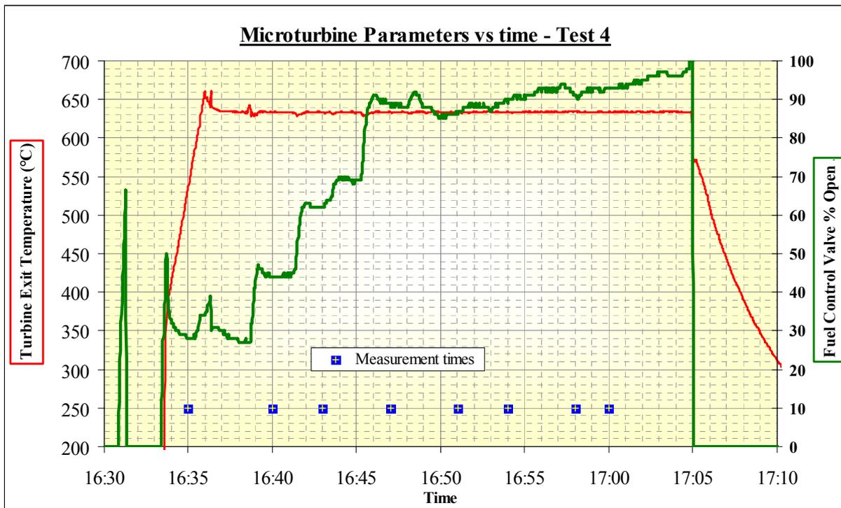
**Figure 17: Logged Microturbine Parameters During Test 4**
