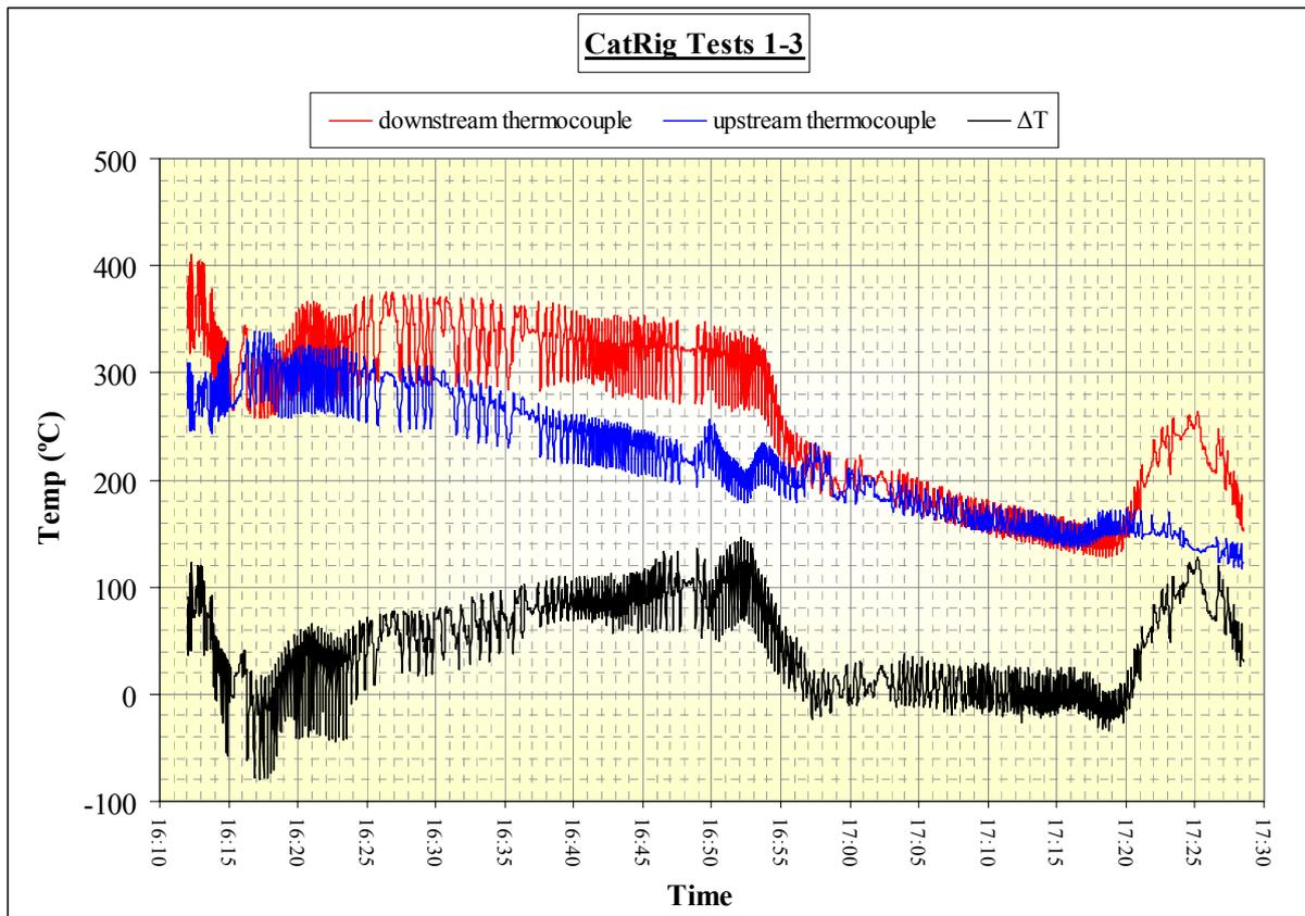
**Figure 40: Temperature record of CatRig Tests 1-3**
