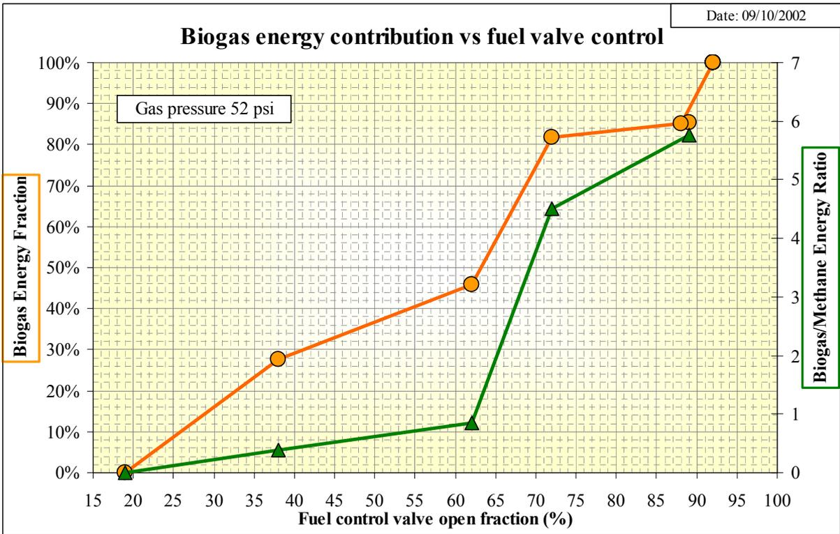
Figure 36: Fuel Energy Balance Analysis in Test 9
