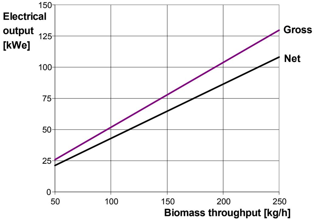
Figure 7. Gross and Net electrical output v's biomass throughput (gasifier efficiency 80%, turbine efficiency 26%, 50% turbine deration)
