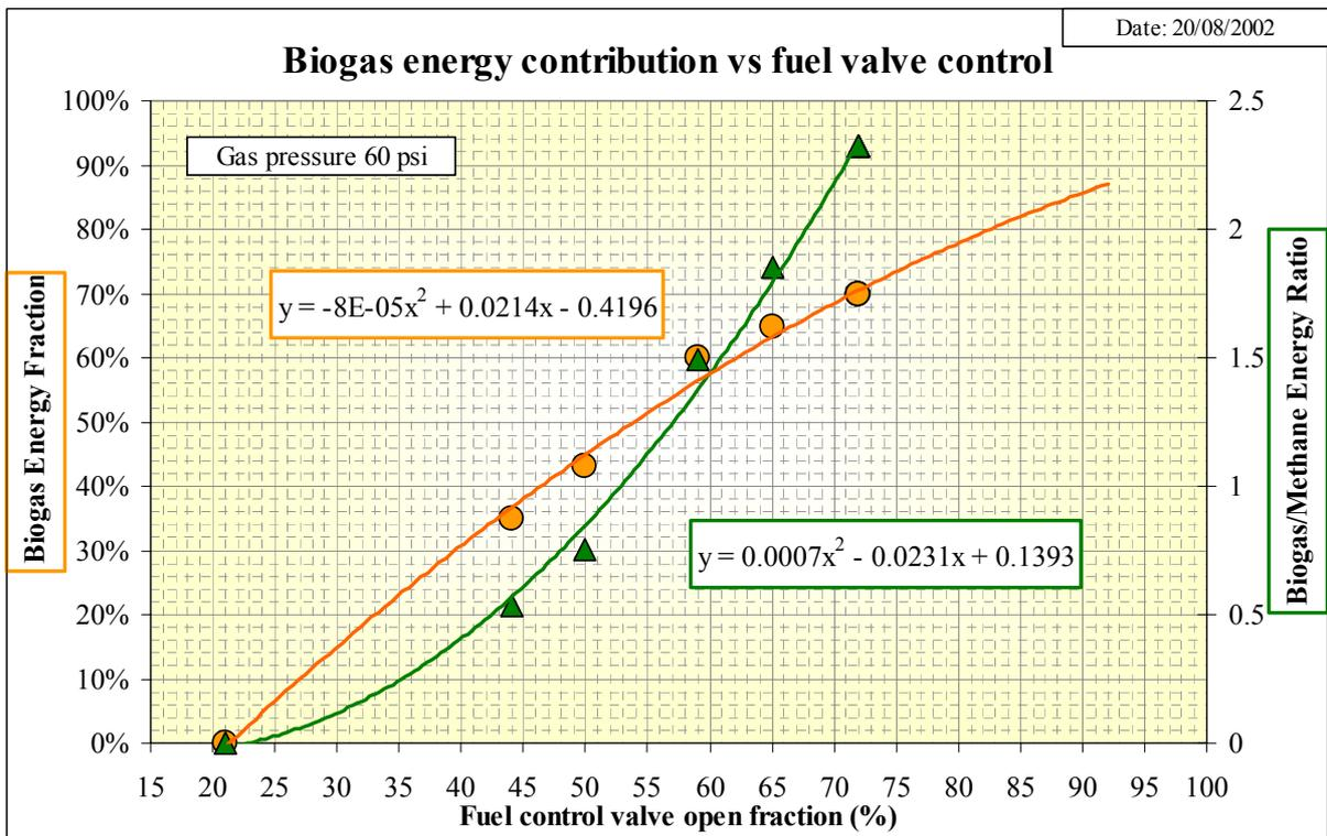
**Figure 16: Fuel Energy Balance Analysis in Test 3**
