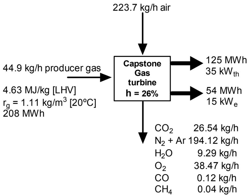
Figure 4. Capstone Gas Turbine Mass Balance
