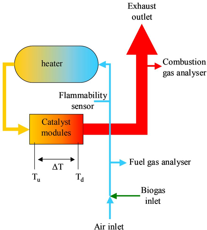
**Figure 38: Side elevation schematic of catalytic combustion test rig**
