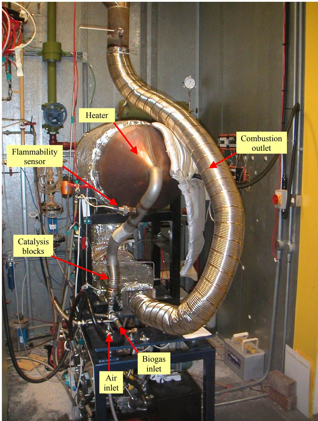
**Figure 39: Photo of the Catalytic Combustion Test Rig in Advantica Test Cell 2**
