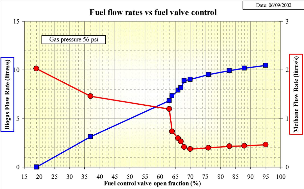
Figure 27: Fuel Volume Flow Rates in Test 7
