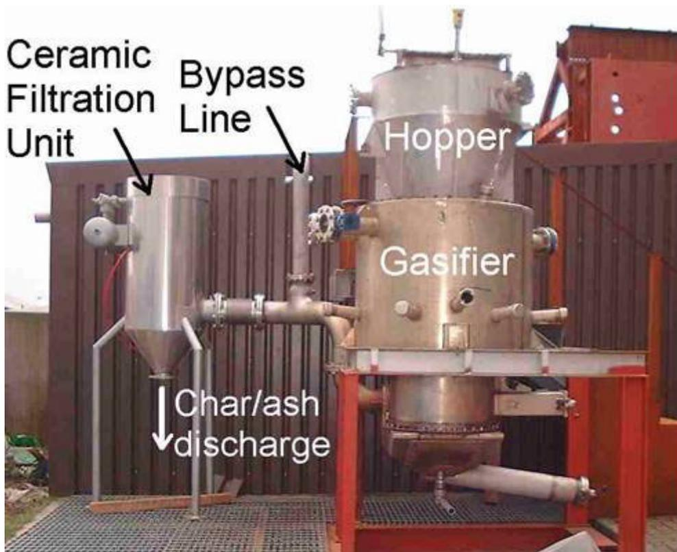
Photograph 1. Gasifier and Test filtration unit without feed conveyor (prior to addition of char/ash bin)
