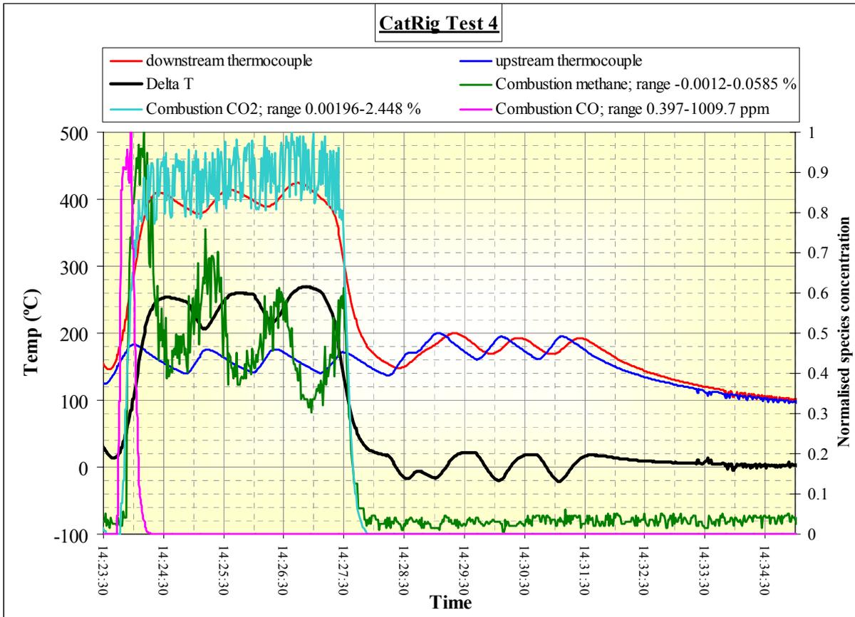
Figure 41: Temperatures and gas species concentrations for CatRig Test 4
