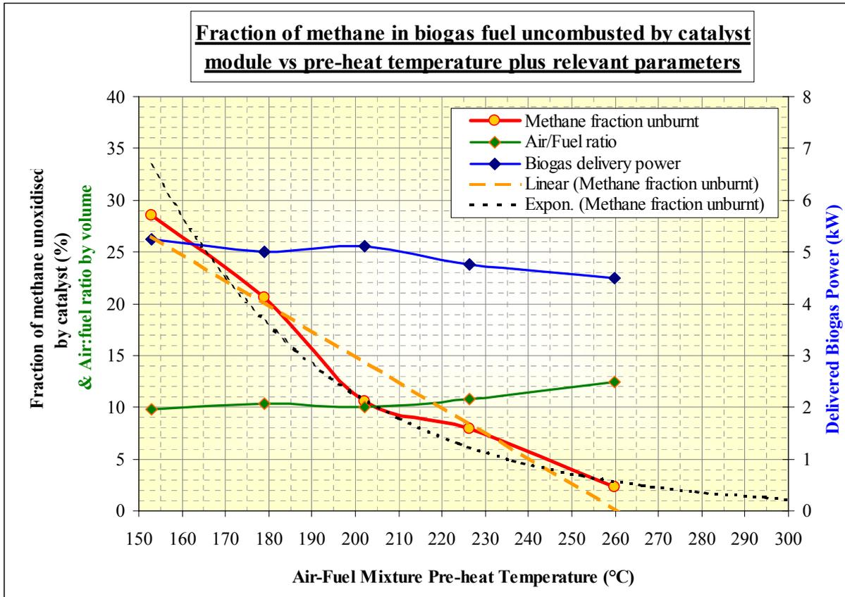
**Figure 44: Dependence of unburned methane fraction on pre-heat temperature**
