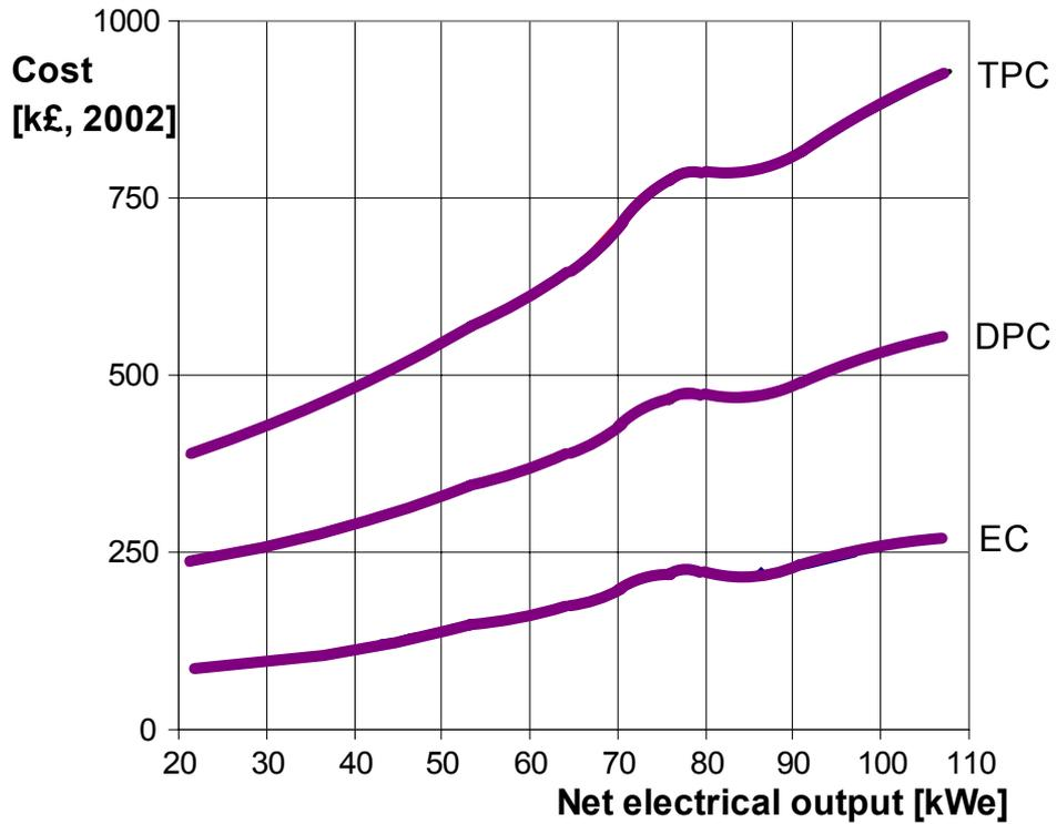
Figure 5. Plant costs: Equipment Cost (EC), Direct Plant cost (DPC) and Total Plant Cost (TPC) v's net electrical output (Model C330 MGT)
