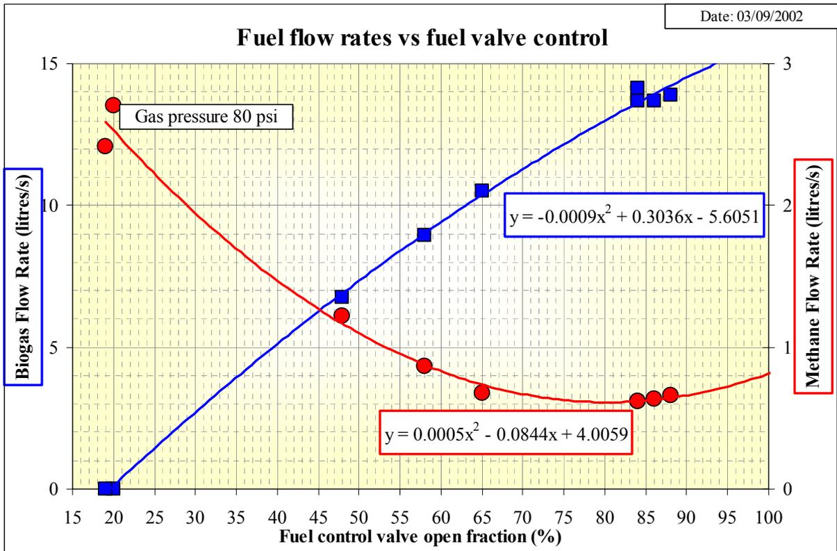
Figure 21: Fuel Volume Flow Rates in Test 5
