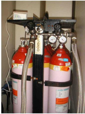
**Figure 30: Synthetic biogas pack after conversion to twin regulator delivery**
