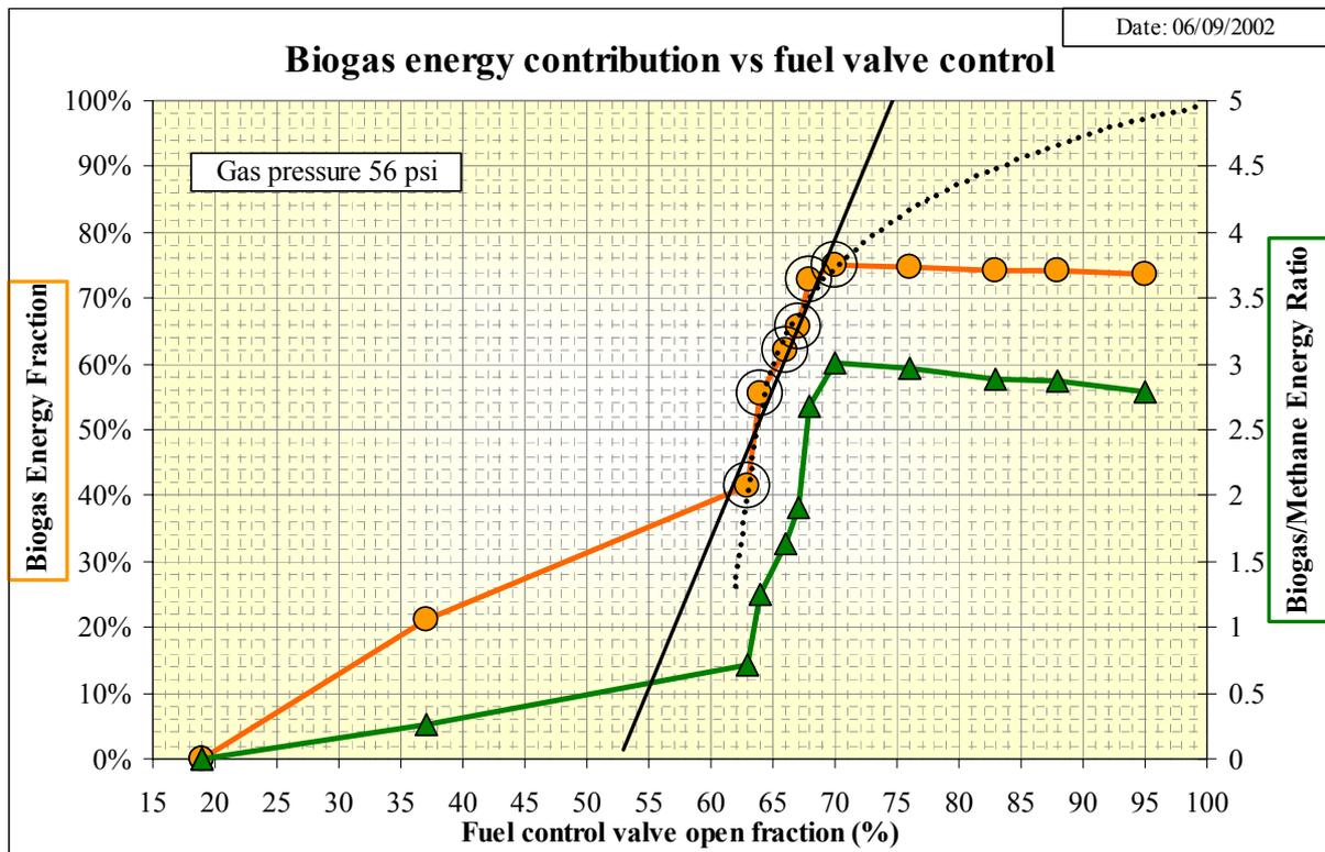
**Figure 28: Fuel Energy Balance Analysis in Test 7**
