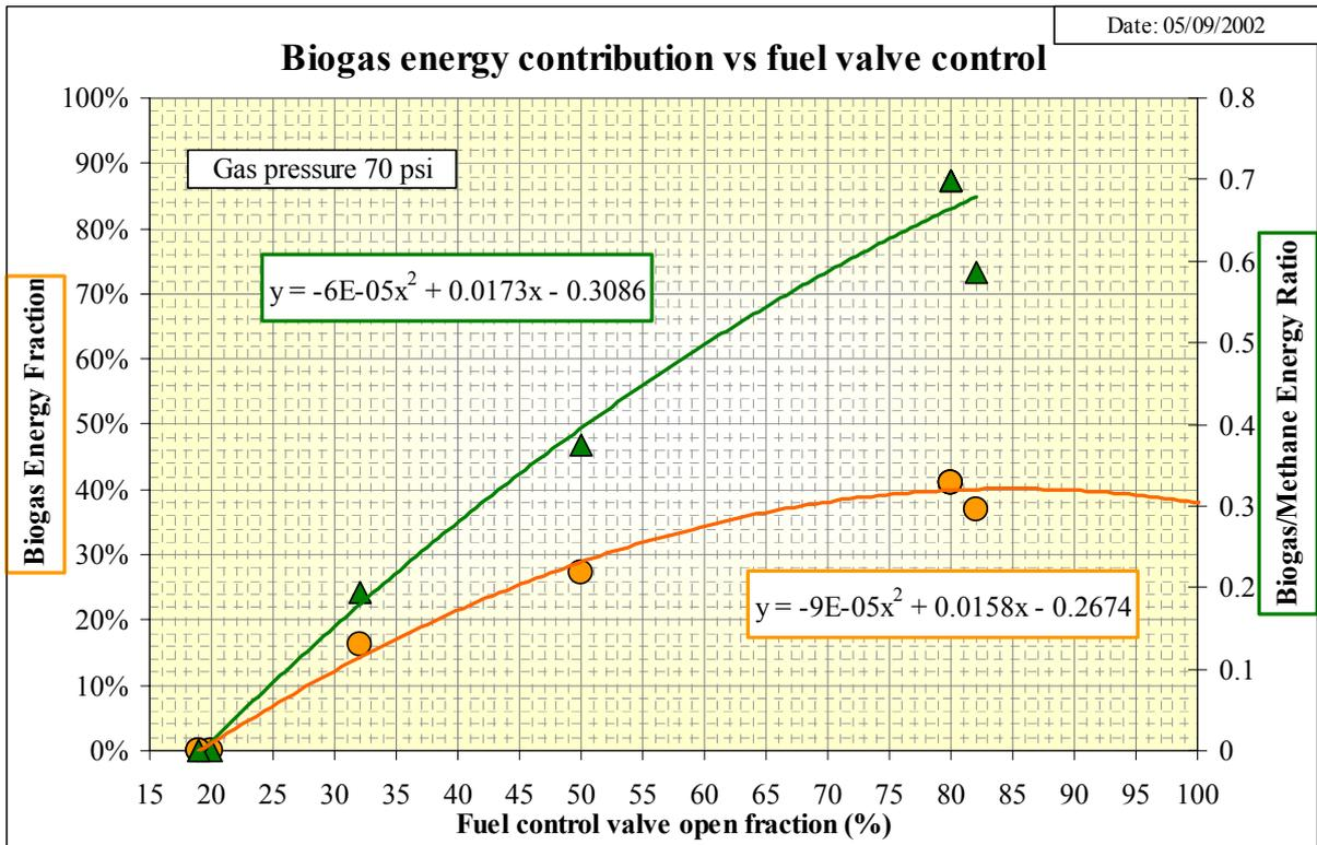
Figure 25: Fuel Energy Balance Analysis in Test 6b
