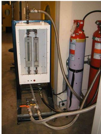
**Figure 29: Gas blender unit after conversion to twin 1" hose biogas delivery &**
