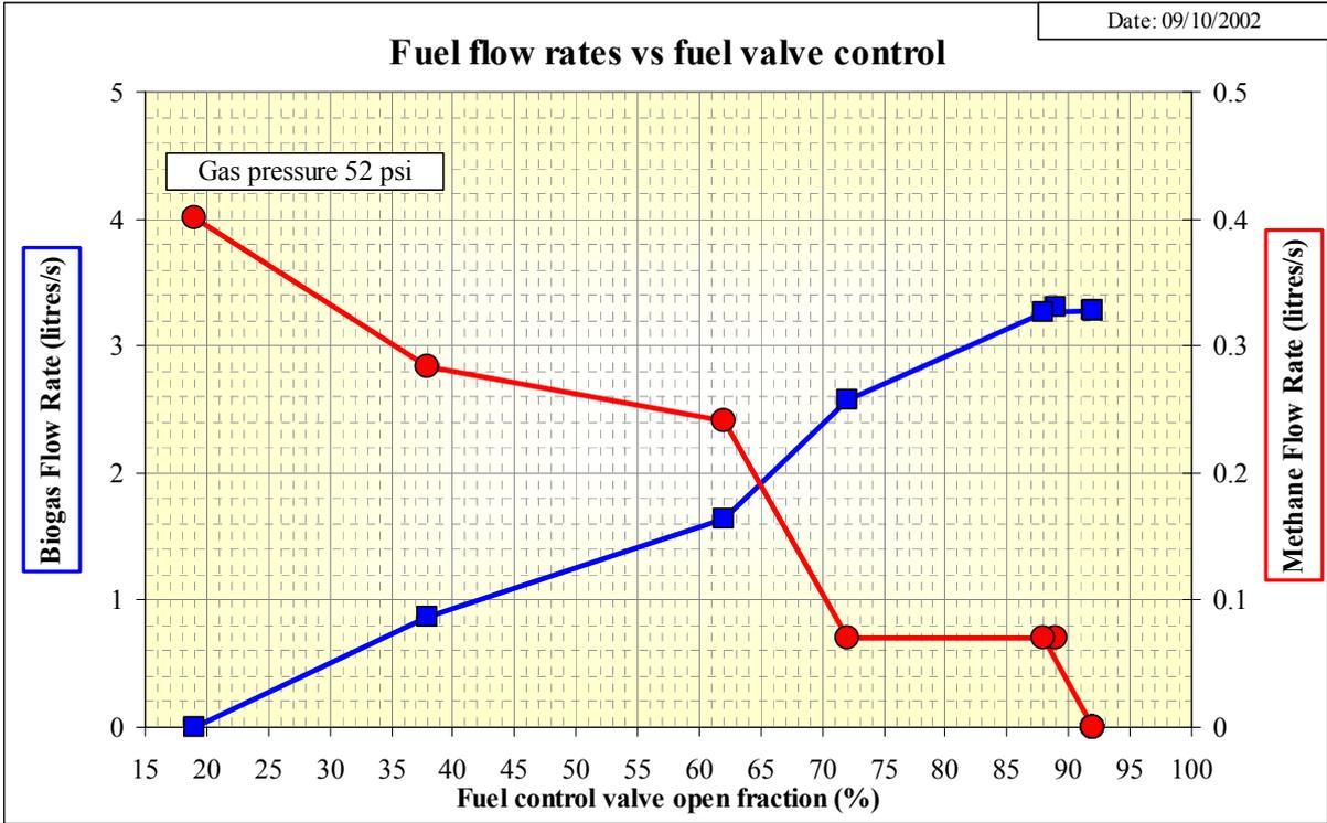
Figure 35: Fuel Volume Flow Rates in Test 9
