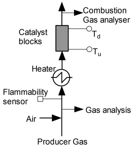
Figure 3. Schematic of catalytic combustor test rig at Advantica
