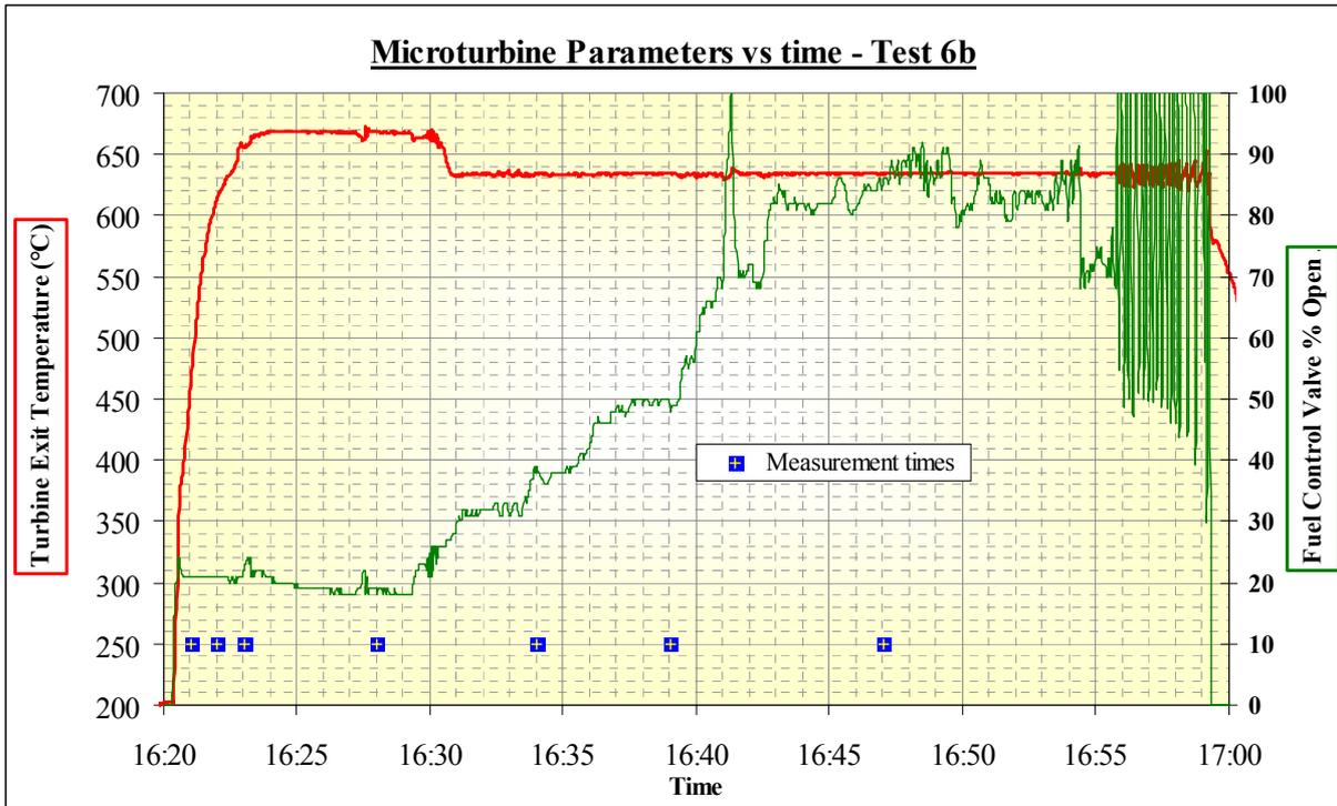
Figure 23: Logged Microturbine Parameters During Test 6b
