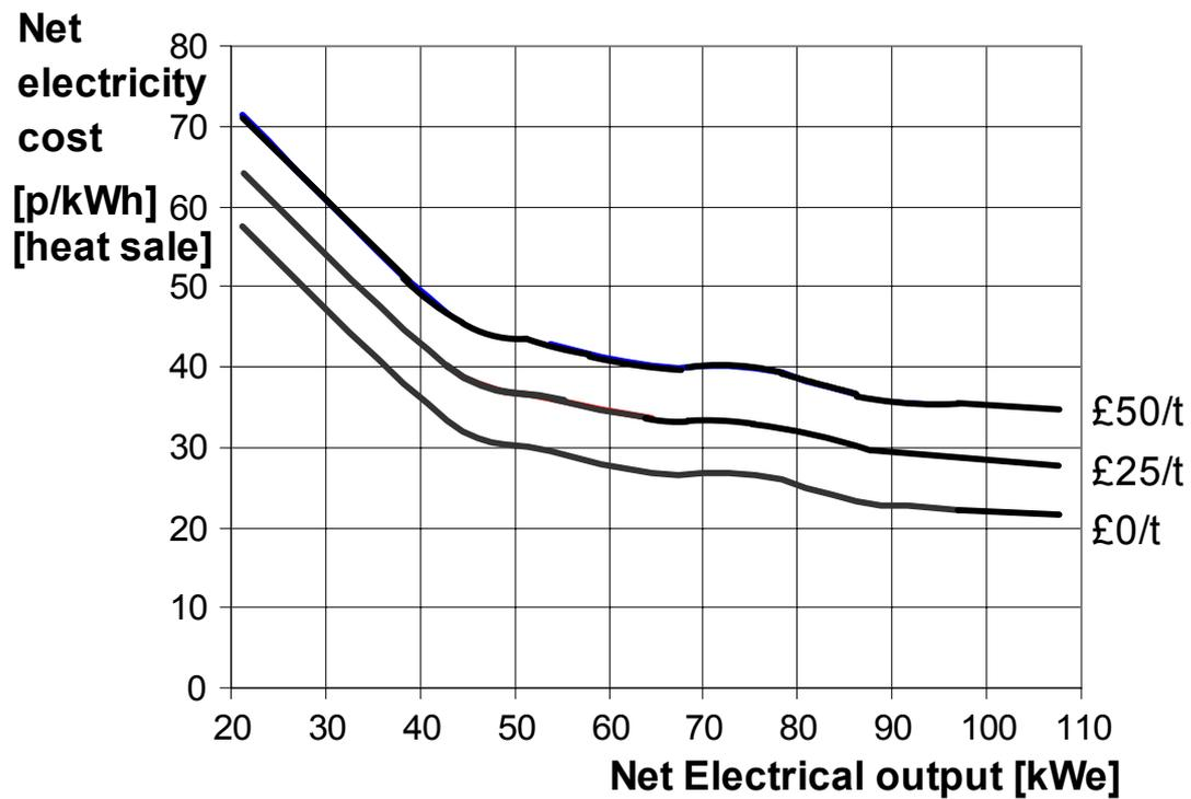
Figure 9. Comparison of net electricity production cost with CHP option – income from heat (1 p/kWh). Variation with feedstock cost
