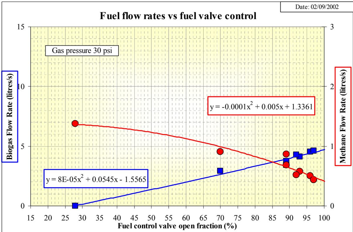
Figure 18: Fuel Volume Flow Rates in Test 4
