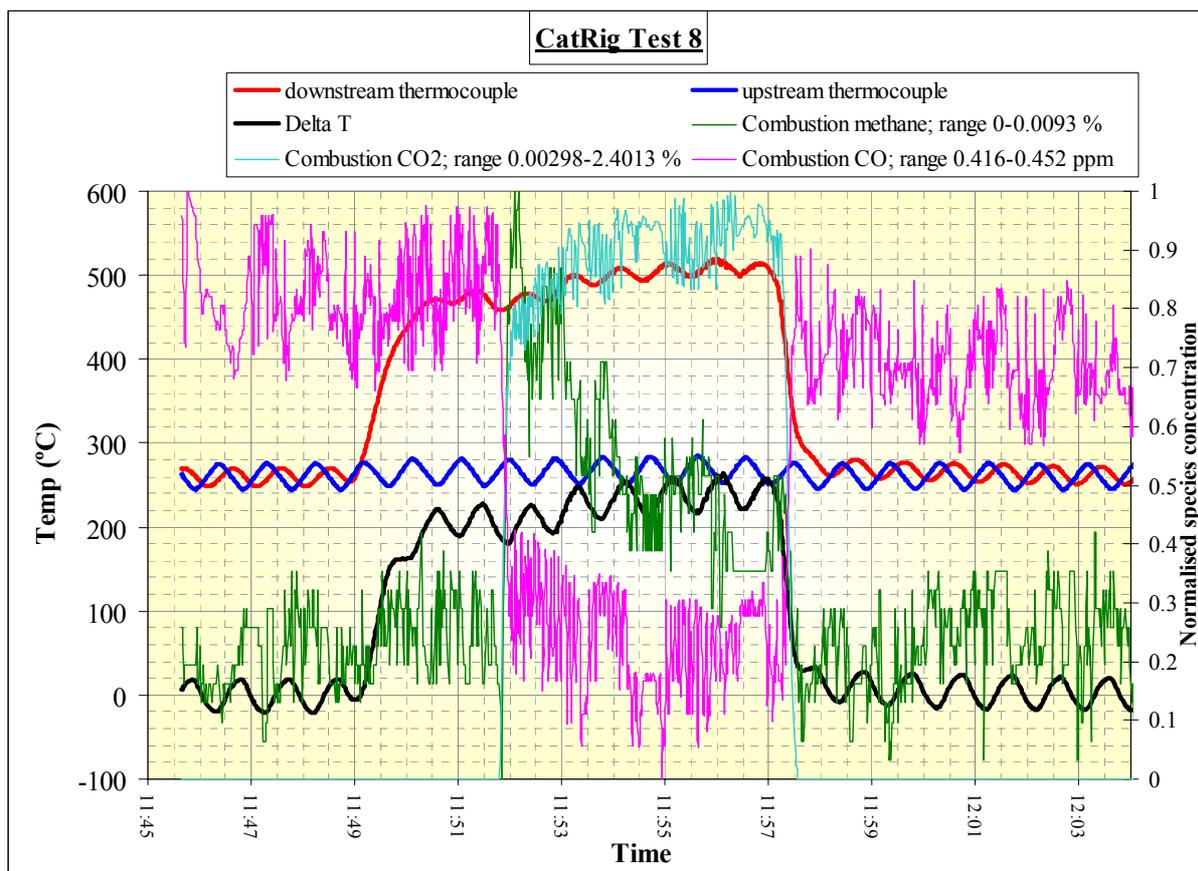
**Figure 43: Temperatures and gas species concentrations for CatRig Test 8**
