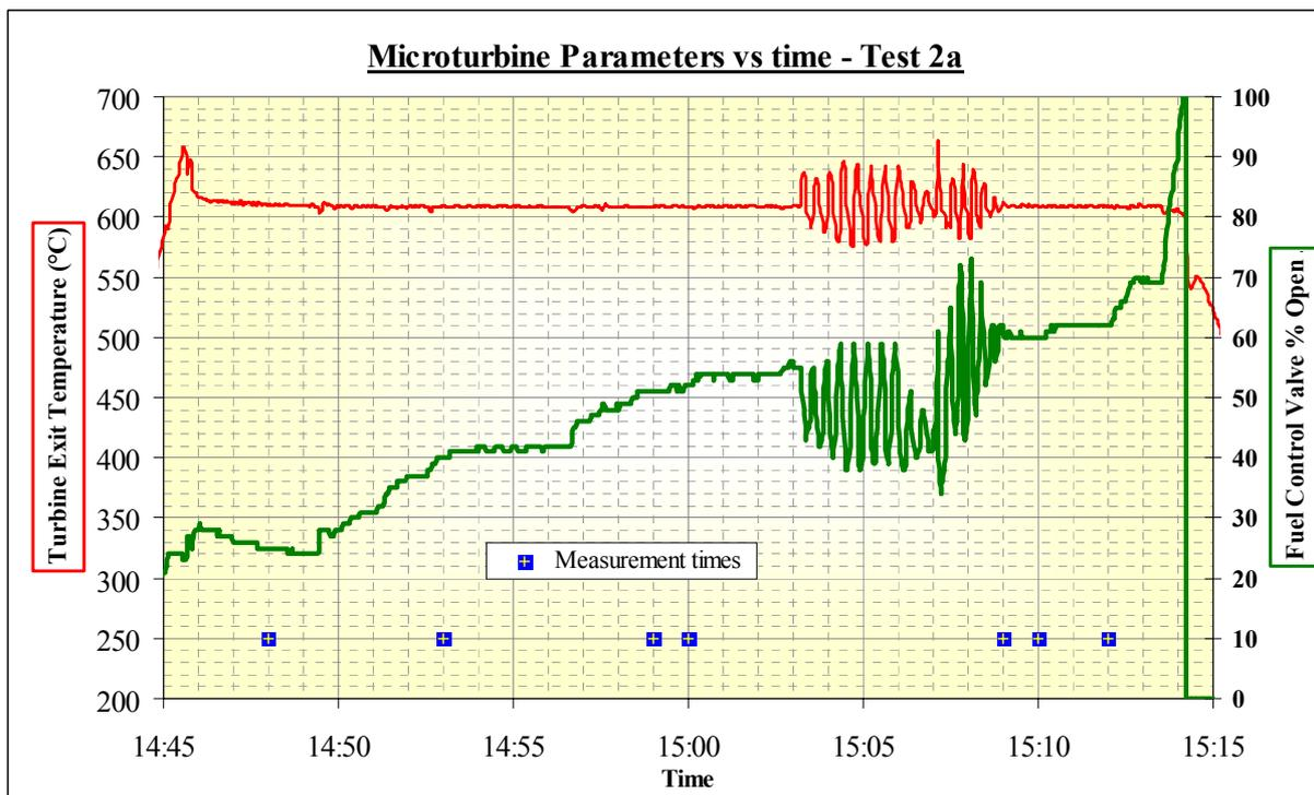
**Figure 11: Logged Microturbine Parameters During Test 2a**
