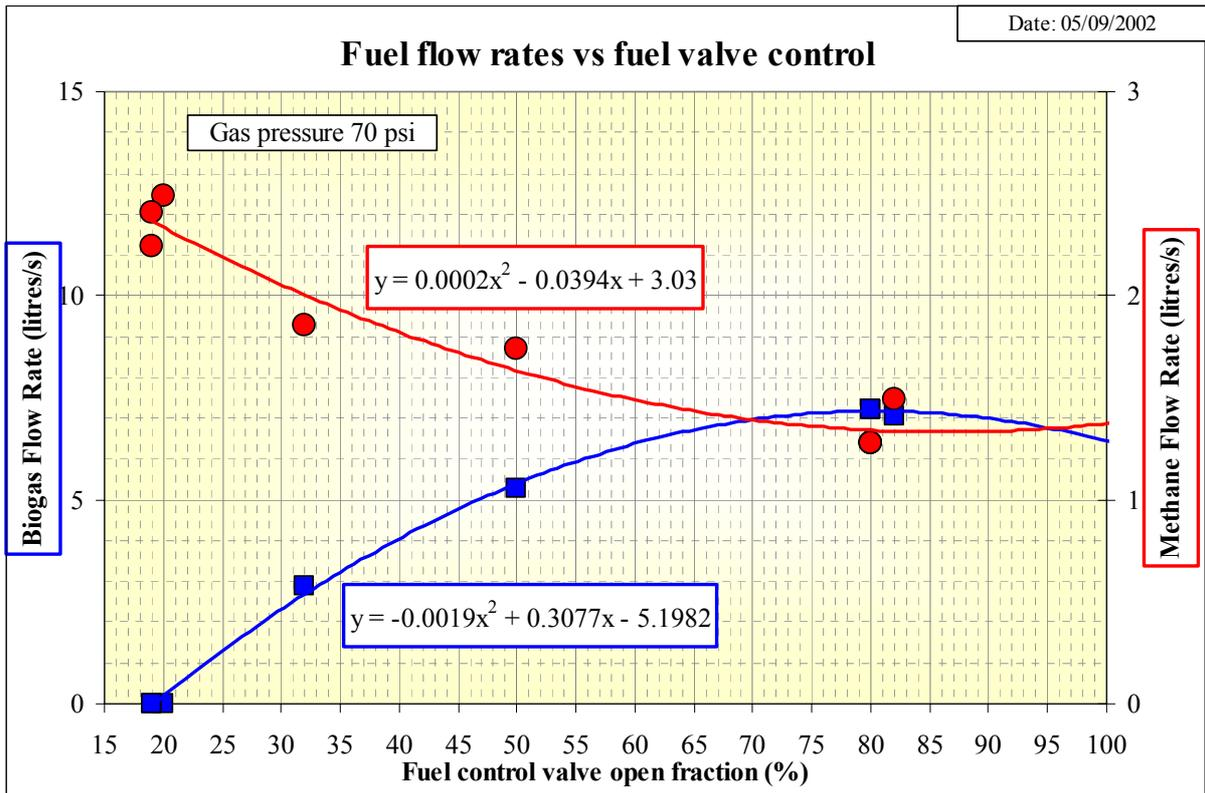
Figure 24: Fuel Volume Flow Rates in Test 6b
