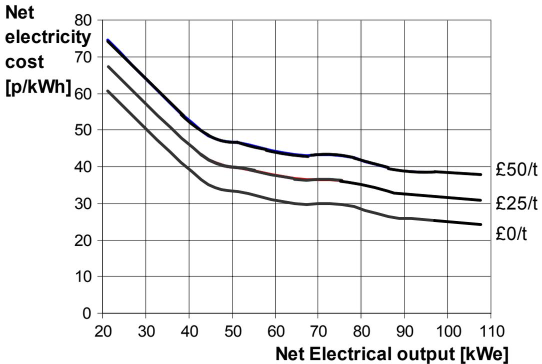
Figure 8. Net Electricity Production cost v's electrical output: variation with prepared feedstock cost
