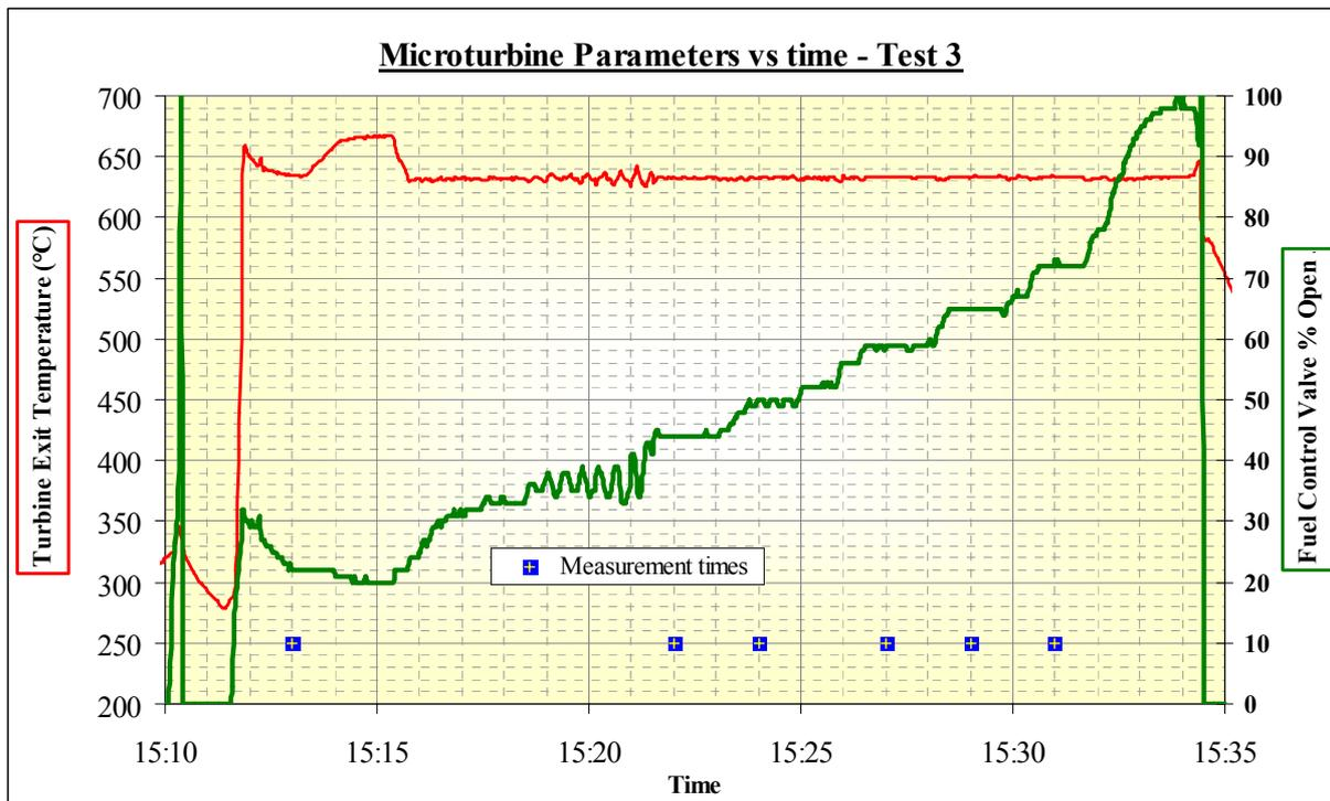
**Figure 14: Logged Microturbine Parameters During Test 3**
