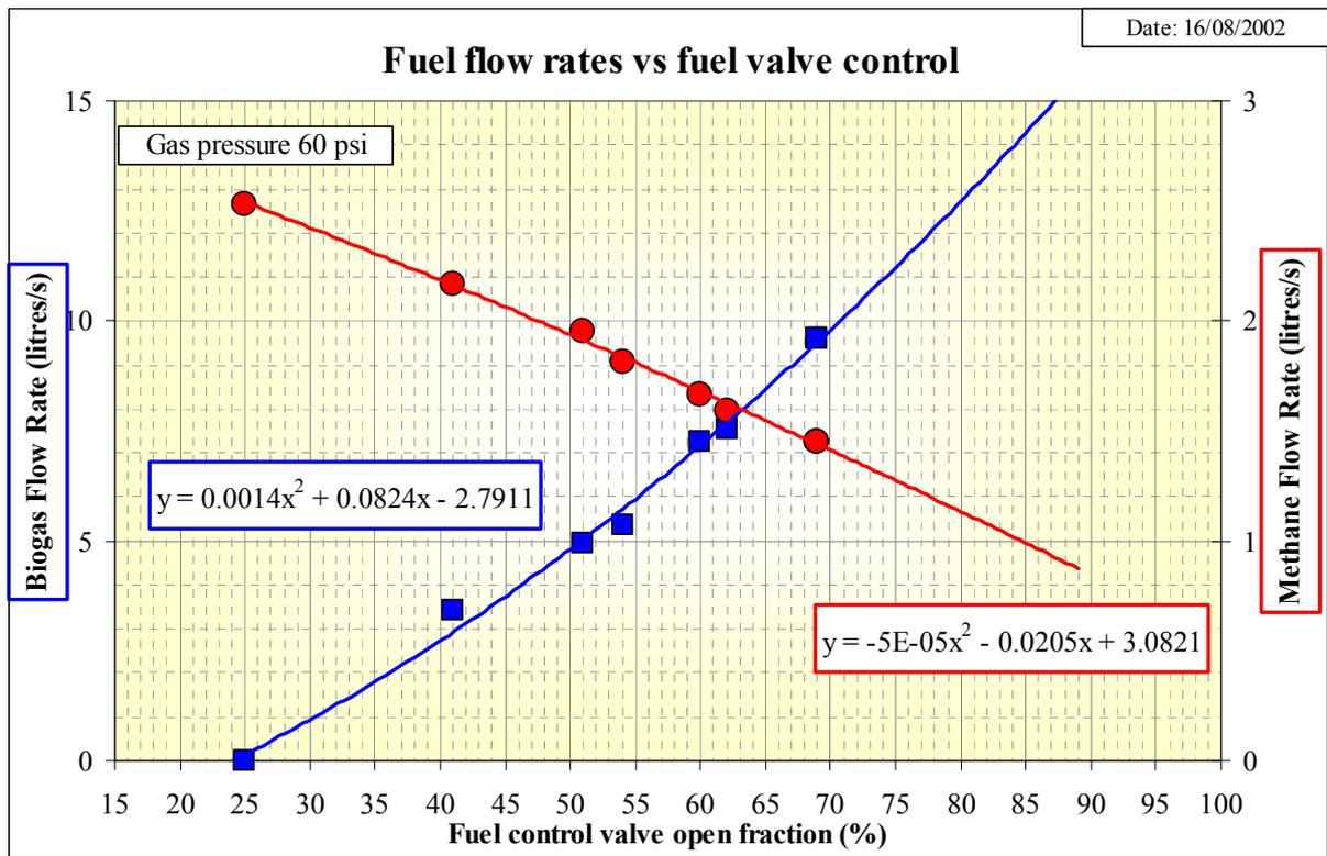
Figure 12: Fuel Volume Flow Rates in Test 2a
